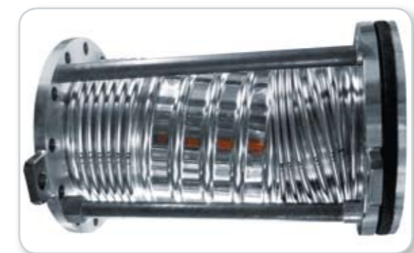
Unsteady deformed bellows caused by internal pressure
